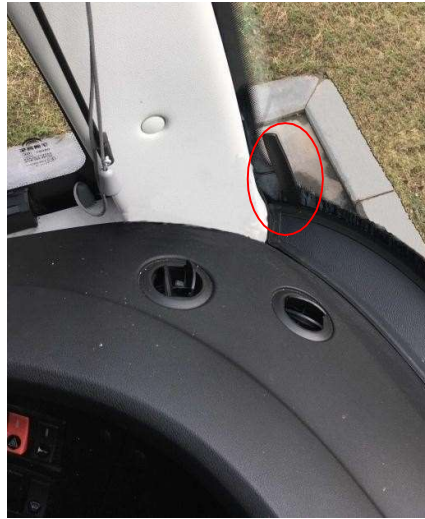
Figure 2-24 Inside installation of Mobile Network Antenna
