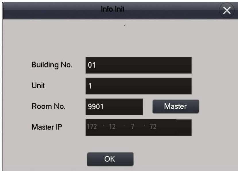
Figure 5-32 Step 4 Initialize the VTH.
