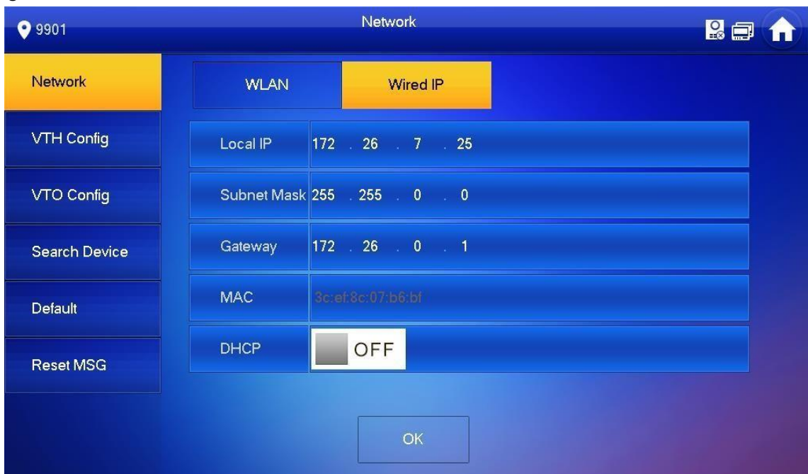
Figure 5-15 Step 4 Set according to actual network access mode.
